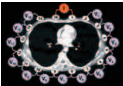
Fig. 2: A first pair of electrodes applies a very small current into the thorax while the remaining 13 electrode pairs measure the resulting voltage signals and their changes.
