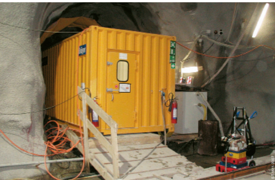
This self-contained rescue chamber protects against smoke and particles.
